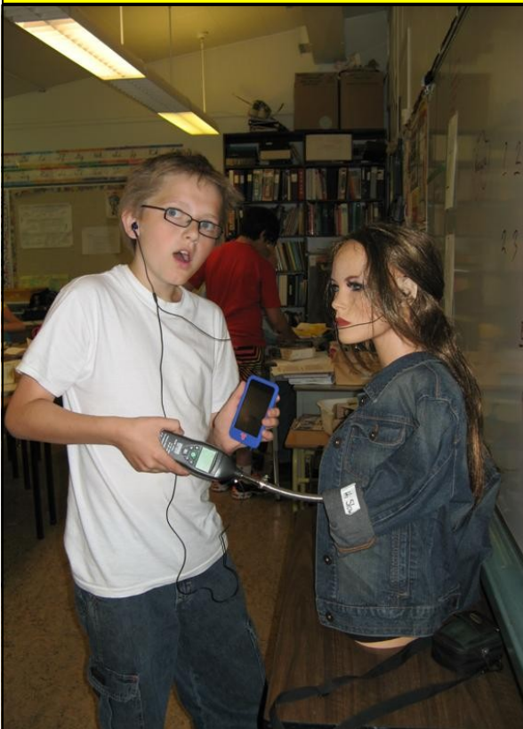
Students at Canyon Lister Elementary and the Alternate School in Kaslo plugged their ear buds into Sasha and found that the volume on their iPods could lead to hearing loss if they didn't turn down the volume. Sasha measures the decibels of music from an iPod and a chart tells us the permissible exposure time at that volume.
